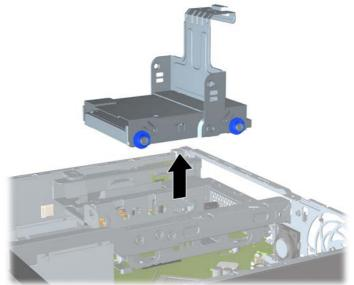
7. Remove the four guide screws from the sides of the hard drive carrier.
